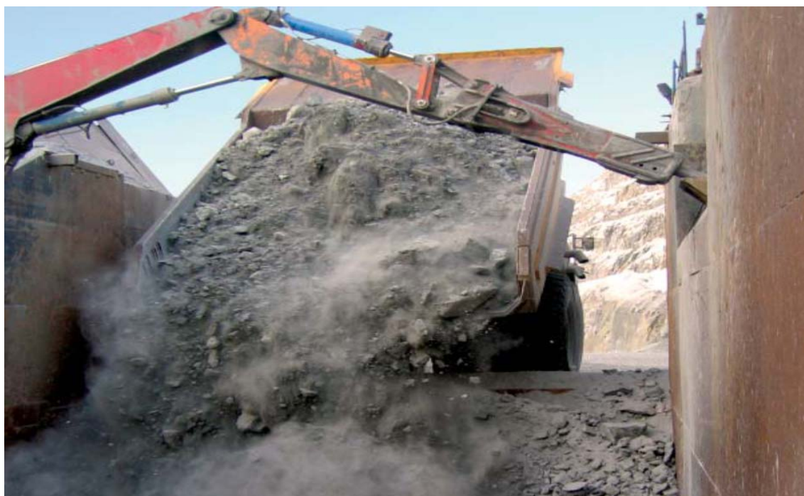
Figur 41. Innlasting i en spindelknuser (gyratory crusher)
