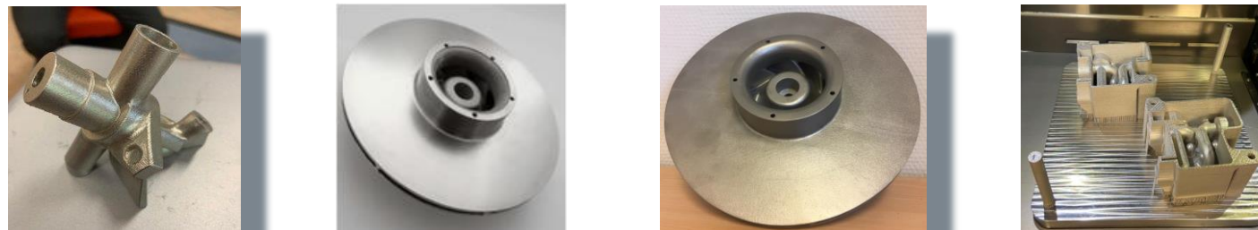
Examples of alloy 718 nozzle holder, impellers in Ti Grade 5 and alloy 625, and hydraulic block in alloy 625 following DNV-ST-B203
