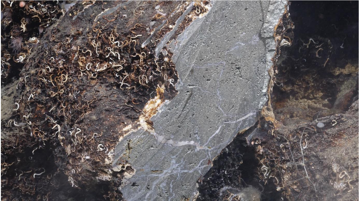
Figure 14: Cut surface of a massive sulfide sample with white veins (calcium carbonate).
