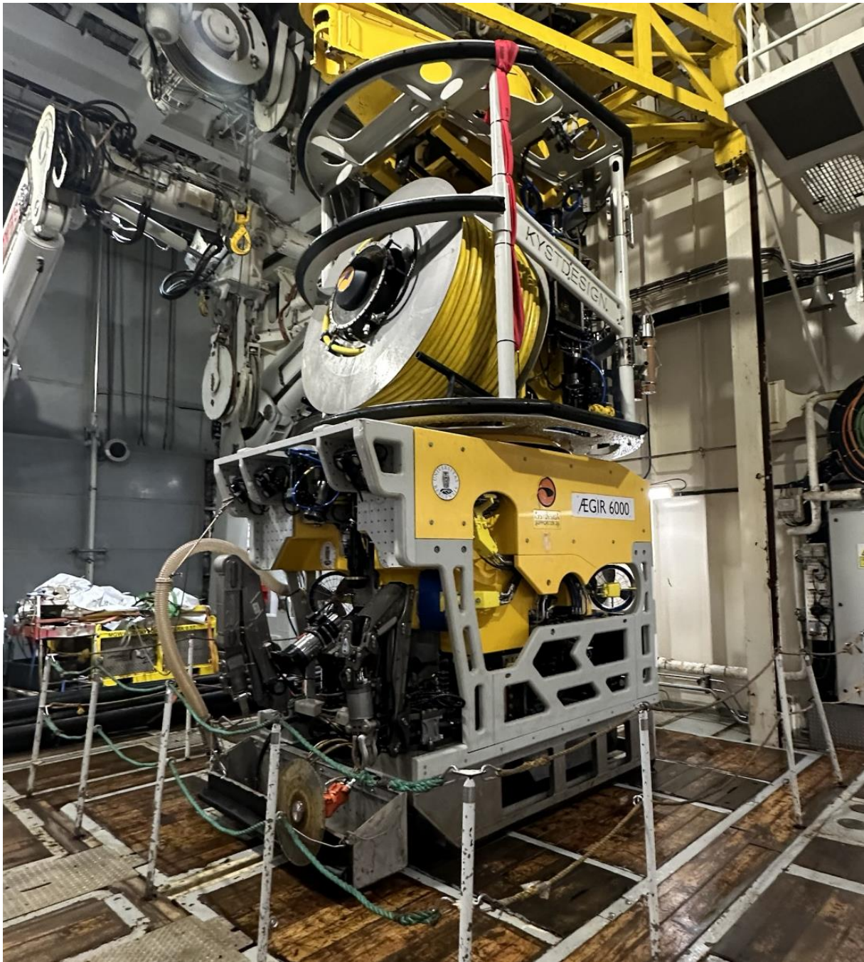
Figure 3: The ROV Ægir 6000 and TMS. Equipped with the saw and suction sampler
