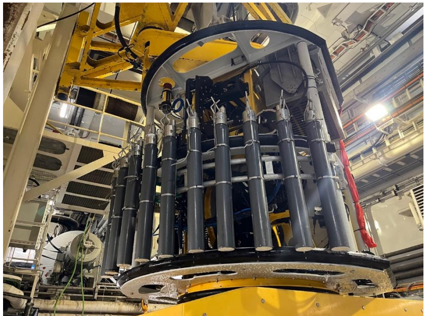
Figure 4: The 10 push cores (A-J) attached to the Tether Management System (TMS) by metallic hose clamps.
