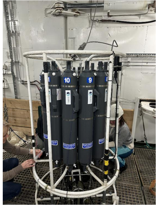
Figure 5: The CTD instrument with 12 Niskin bottles for water sampling.
