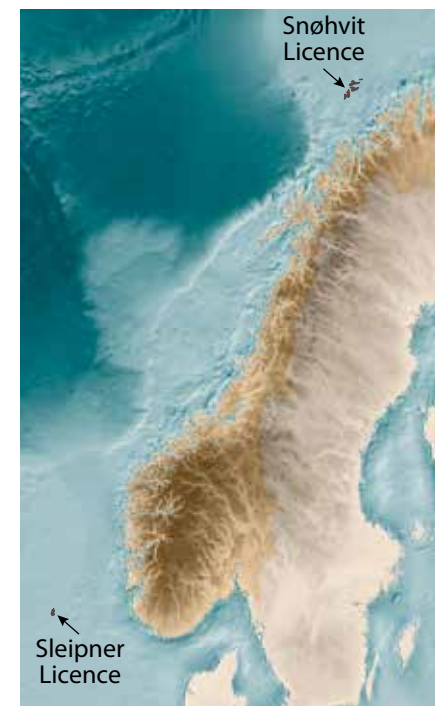
Snøhvit: There is capacity for separation and storage of 700 000 tonnes annually in water saturated sandstone reservoirs under the Snøhvit Field in the Barents Sea. A shale cap which lies above the sandstone will seal the reservoir and ensure that the CO 2 stays underground.
