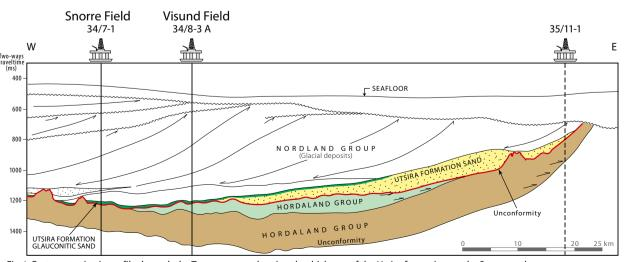
Fig 4: East-west seismic profile through the Tampen area, showing the thickness of the Utsira formation on the Snorre and Visund fields. The location of the profile is shown in fig 3.
