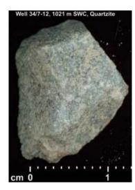
Fig 5: Sharp-edged quartzite stone found in a sidewall core close to the base of the unit interpreted by Statoil as the Utsira formation. This piece of rock hails from the mainland and must have been carried to the Tordis area during the ice age – long after the Utsira was deposited.
