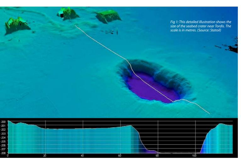
Stratigraphic studies by the NPD in the wake of an oil leak on Tordis have shown that the Utsira formation is not present where an injection well was drilled for this North Sea field.
