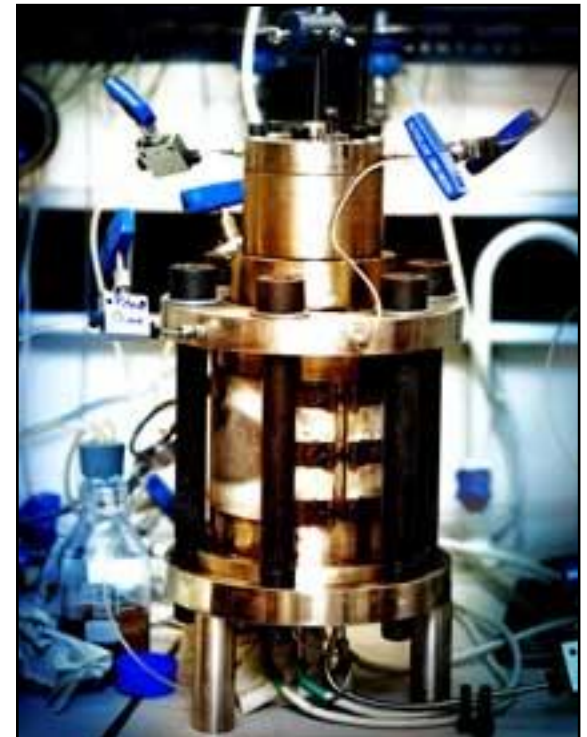
Triaxial cell, 130 °C, ca. 12 MPa stress
