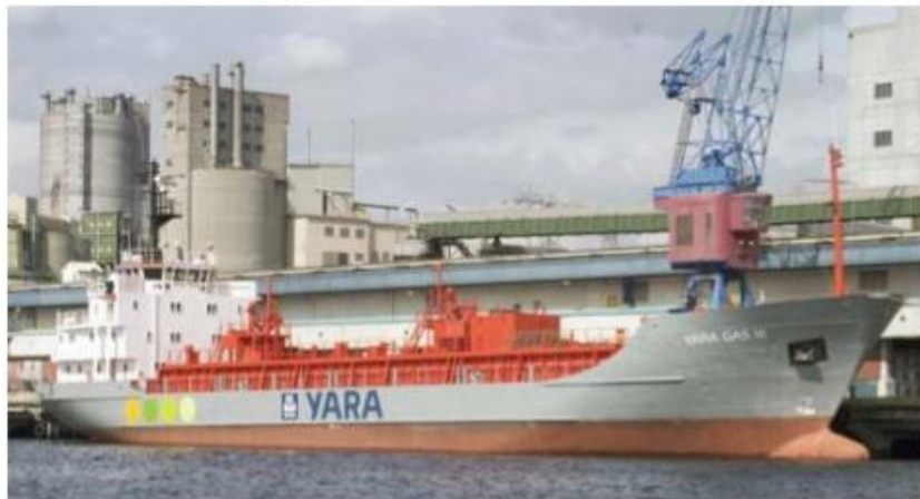
M/T Yara Gas III alongside the quay near Yara's ammonia plant in Porsgrunn, Capacity: 1200 t of liquefied CO 2 in 2 tanks of 600 tons capacity each Ship type: Converted container vessel
