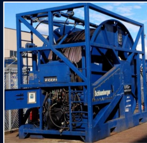
Coiled Tubing carrying optical fibers
