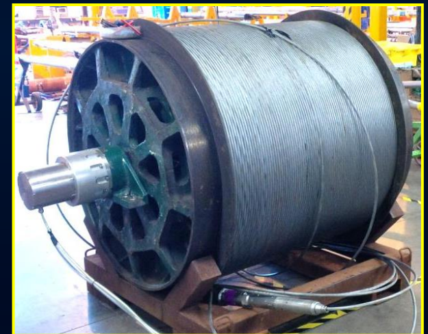
Hybrid Wireline Logging cables Coaxial and heptacables
