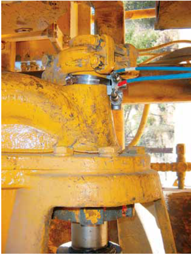
Figure 7-15. Accelerometers mounted on the auxiliary entry port of the gooseneck on the topdrive unit of the rig at San Andreas Fault Observatory at Depth (SAFOD). This is the preferred mounting position: directly above the drillstring and as close as possible to the host pipe in the drillstring.
