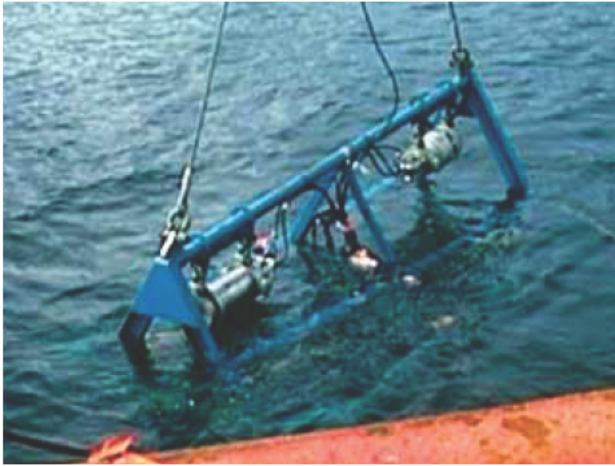
Figure 3-11. High-performance Magnum six-gun array. (Picture from North Sea operations.)
