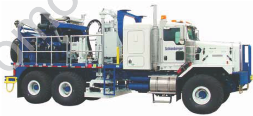
Figure 3-17. The Schlumberger latest generation of truck-mounted vibrator, with 60,000 lbf peak force.
