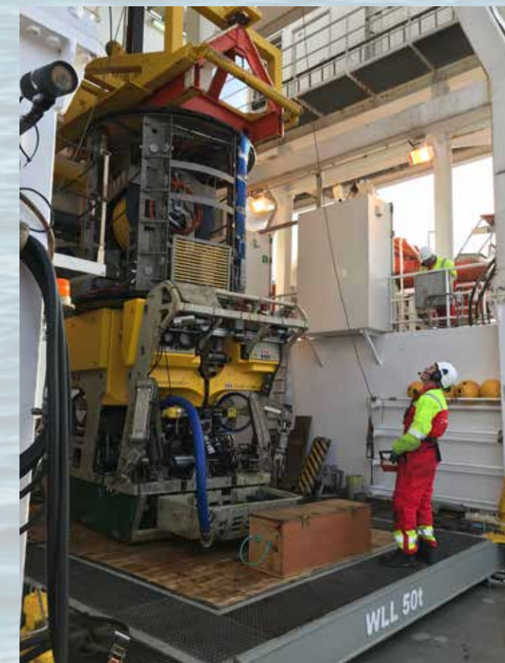
ROV A remotely operated vehicle (ROV) is one of the tools used for subsea mapping and sampling. (Photo: K G Jebsen Centre for Deep Sea Research, University of Bergen)
