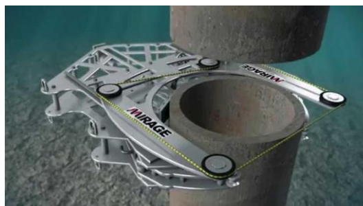
> Figur 10-14: Diamant wiresag for undervanns stålkutting [86]
