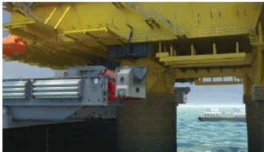
3. The active motion compensation system is engaged
